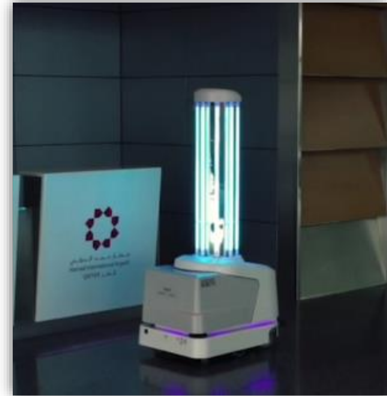
Fully autonomous mobile disinfection robot
